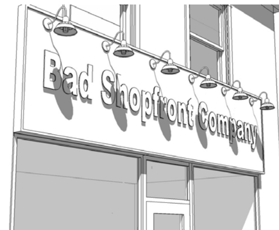
Figure 8– Poor lighting scheme that dominates the fascia
