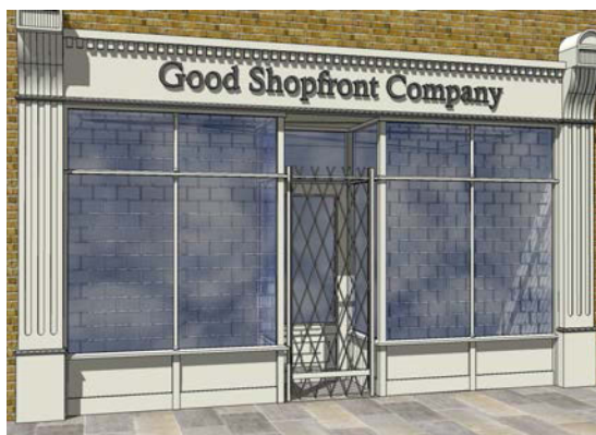
Figure 13– Internal/ external grille arrangement for recessed door
