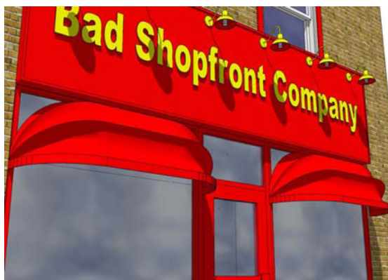
Figure 15– Fixed canopies are often inappropriate.
