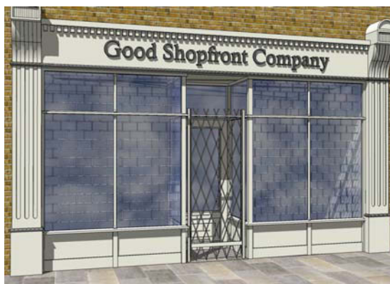
Figure 13– Internal/ external grille arrangement for recessed door
