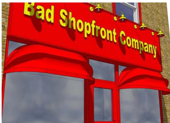
Figure 15– Fixed canopies are often inappropriate.
