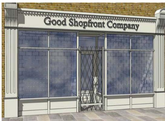
Figure 13– Internal/ external grille arrangement for recessed door
