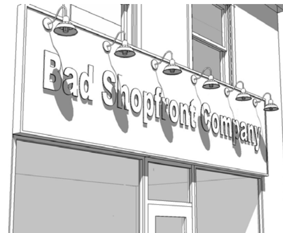
Figure 8– Poor lighting scheme that dominates the fascia
