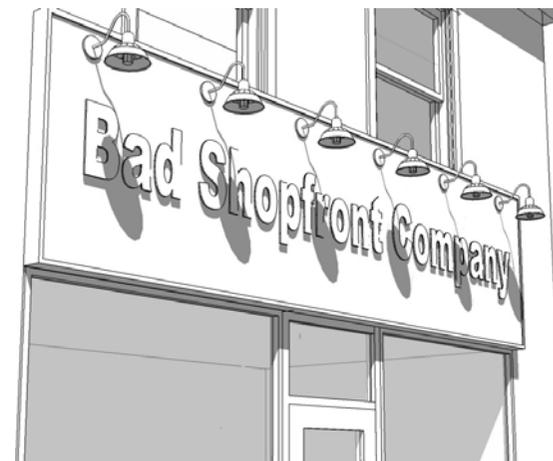
**Figure 8– Poor lighting scheme that dominates the fascia**
