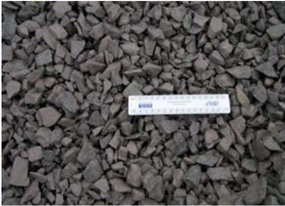
Permeable subbase (4/20 material)
