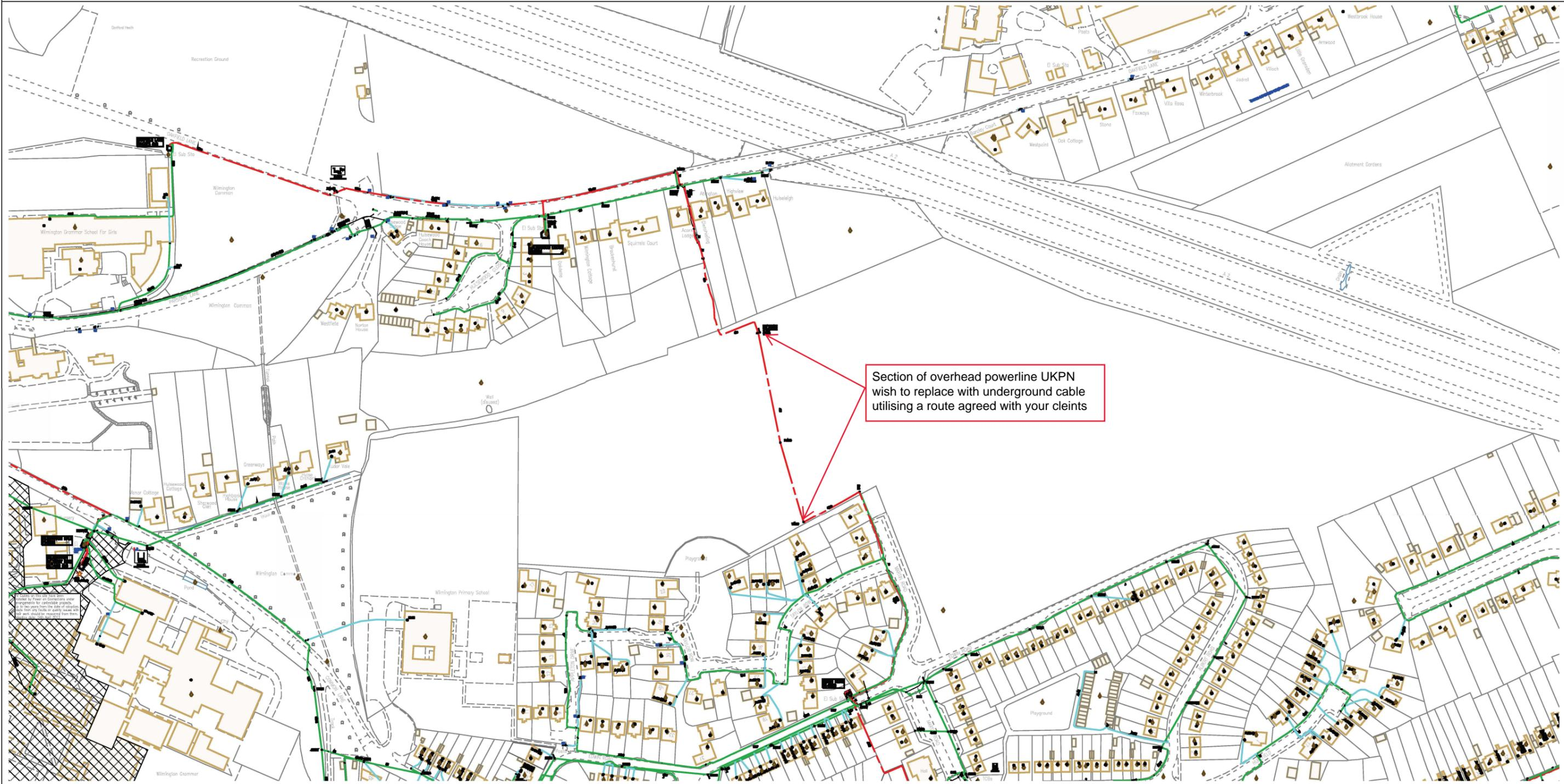
Section of overhead powerline UKPN wish to replace with underground cable utilising a route agreed with your clients
